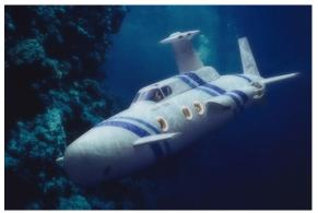
support for a dozen passengers, built-in air-conditioning, and up to eight tons of payload. It can run at speeds of up to 11 knots on the surface, as well as 15 knots when submerged in the water.
