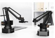
objects for you), and a laser engraving kit, each of which can be attached to the head to accomplish any desired tasks. For control, it can be manually operated either via mouse-and-keyboard or a companion mobile app, as well as programmed using a graphical interface based on Blockly. It can also learn movements by physically moving the arm, as it can remember motion sequences and repeat it when triggered.
