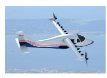
became the first to break the speed of sound. The innovation that's been synonymous with the designation continues with the agency's first X-plane in over a decade: the NASA X-57 Maxwell, the first one to rely exclusively on electric motors for power.
